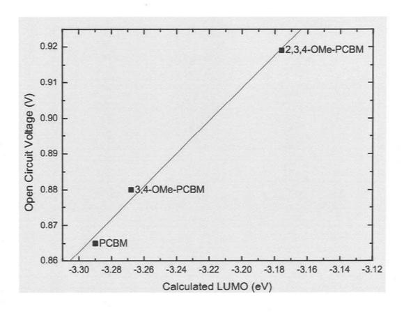
Figure 6: Open circuit voltage of MDMO-PPV: fullerene devices [21] versus theoretical LUMO levels (B3LYP/3-21G\*) of acceptors for blend film dissolved in chlorobenzene.
