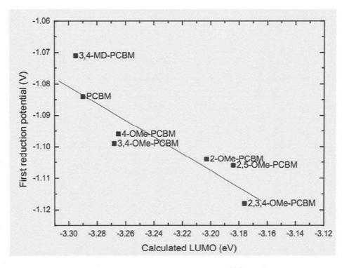
Figure 5: First reduction potentials of fullerene derivatives [21] versus LUMO levels calculated with DFT B3LYP/3-21G\* level of theory.
