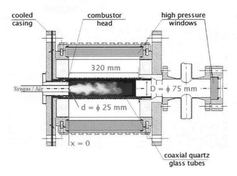
Figure 1: Sketch of the experimental dump-combustor test rig.
