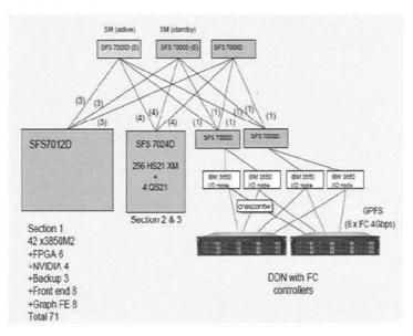
Figure 2: Architecture of the InfiniBand network including the IBM/DDN 9550 storage system. The 4 I/O Nodes, directly Fibre Channel attached to the storage are the GPFS NSD servers.
