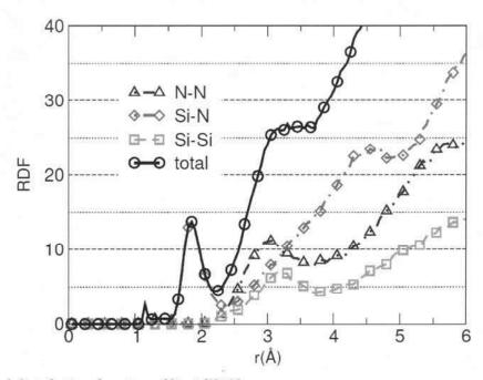
Figure 4: Radial distribution function of liquid Si<sub>3</sub>N<sub>4</sub>
