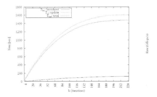
Figure 4: At k-th iteration the ratios  $T^{acc}_{bc}(k)/T^{acc}_{tot}(k)$  and  $T^{acc}_{up}(k)/T^{acc}_{tot}(k)$  are roughly constant. The figure reports the total accumulated time in all of the steps as function of iterations k. We have checked that a such pattern is independent by problem size and number of processes. In the figure is not reported the fraction of time for the panel factorization, that is  $T^{acc}_{lof}(k)/T^{acc}_{tot}(k)$ .
