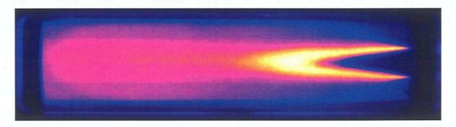
Figure 3: Averaged OH field obtained by using 400 OH-PLIF samples.
