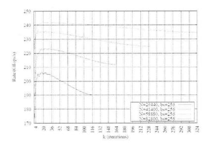
**Figure 7:** The same tests as Fig. 5 respect N but keeping bs = 256 constant. For  $k_{min} = 9$  we obtained the same qualitative trend as reported in Fig. 6. The differences after the maximum value are because load imbalance.
