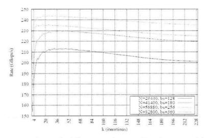
**Figure 5:** The figure shows the trend of flops execution rate (Rate is expressed in Gflops/s) for all iterations k. Are reported various problem size and the block size is chosen to have N/bs constant. The results were obtained using p = 32 cores and  $P \times Q = 4 \times 8$  on Sect.2 cluster, although analogous behaviour of flops rate is found in Sect.1 cluster and AMD cluster.
