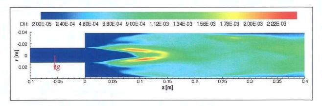
Figure 6: Average OH mass fraction field obtained with the POLIMI chemical mechanism.
