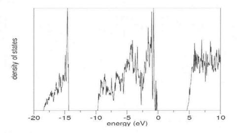
Figure 3: Total electronic density of states of  $\alpha$  Si<sub>3</sub>N<sub>4</sub> material.
