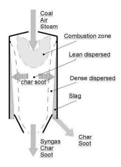
Figure 1: Schematic diagram of the entrained-flow gasifier.
