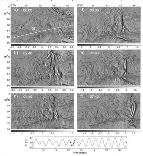
**Figure 3:** From a) to f) Time evolution of surface zonal velocity gradient (in  $10^3$  s<sup>-1</sup>) during the flood tide.  $S_1$  indicates longitudinal cross-section mentioned in Figure 4. Bottom: barotropic tidal transport during the time-series.
