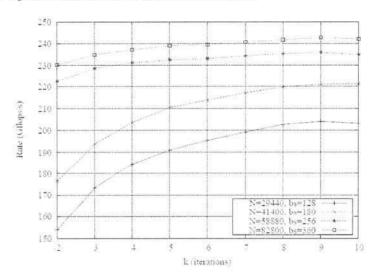
Figure 6: The same HPL tests as Fig. 5 but runs are cut-off at  $k_{min} = 9$  (see condition of eq. (7)). The broadcast topology used is the ring modified.
