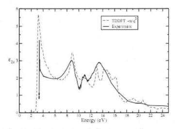
Figure 4: ZnO dielectric function. Experimental results for the extraordinary component, compared with the TDDFT calculations.
