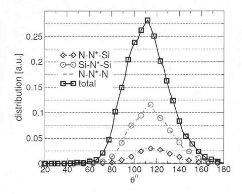
Figure 5: Angular distribution of liquid Si<sub>3</sub>N<sub>4</sub>
