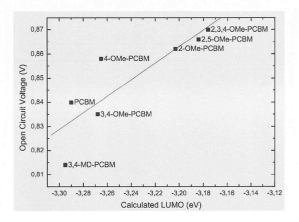
Figure 7: Open circuit voltage of MDMO-PPV: fullerene devices [21] versus theoretical LUMO levels (B3LYP/3-21G\*) of acceptors for blend film dissolved in o-dichlorobenzene.
