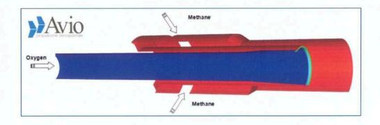
Figure 1: Injector geometrical configuration.
