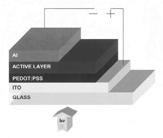
**Figure 1**: Schematic device structure of a polymer/fullerene bulk heterojunction solar cell. The active layer is sandwiched between two contacts: an indium-tin-oxide electrode coated with a hole transport layer PEDOT:PSS and an aluminium top electrode.
