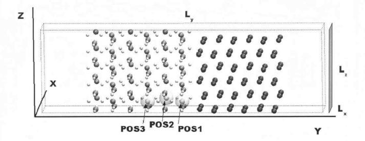
Figure 1: Schematic of the  $MgH_2$ -Mg interface in the simulation box. The structure is infinitely extended in both x and z directions. Free surfaces and  $MgH_2$ -Mg interface are perpendicular to the xy plane. H atoms are in white, Mg atoms are in grey (light grey for Mg in the hydride side and dark grey for magnesium crystalline side). POSx indicates those Mg atoms that are substituted by a Fe atom to study the effect of the catalyst at different distances from the interface.
