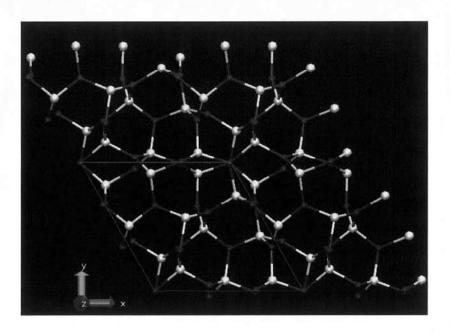
Figure 1: Atomic structure of  $Si_3N_4$  material in its crystalline  $\alpha$  phase. Spheres are the atoms and segments indicates the nearest neighbors atoms of each atom.
