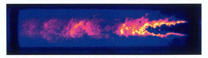
Figure 2: Instantaneous OH field obtained by means of OH-PLIF.
