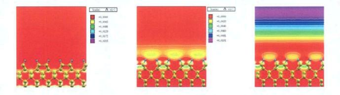
**Figure 1**: From left to right: square modulus of the electronic KS wave function  $|\psi(r)|$  of the HOMO, LUMO and LUMO+1 states at the  $C(0\ 0\ 1)2\times 1$ : H surface. The LUMO+1 state has a NFE character.
