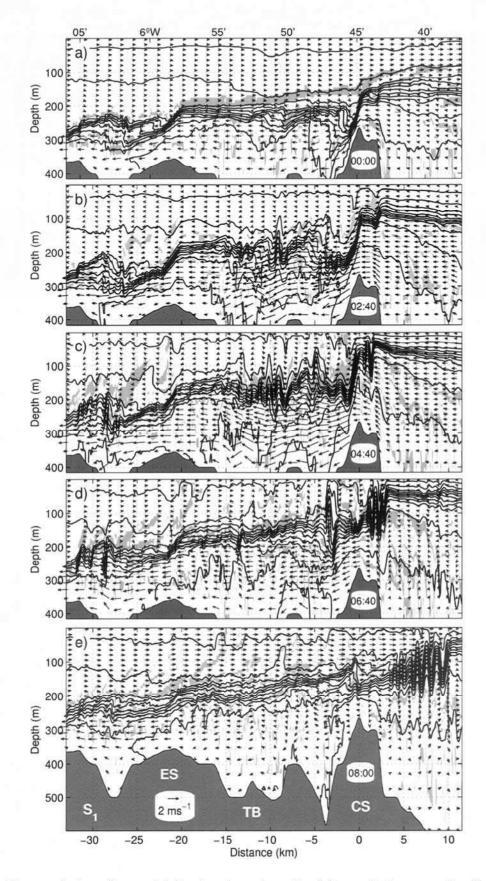
Figure 4: Time evolution of potential density along the axis of the strait (cross-section  $S_1$  in Figure 3). Isopycnal contours 26.80,27.05,...,28.80,29.02 are shown in the figure. Arrows indicate local current velocity. Gray contours indicate areas where Ri < 1/4 and intense water mixing and energy disspation take place.
