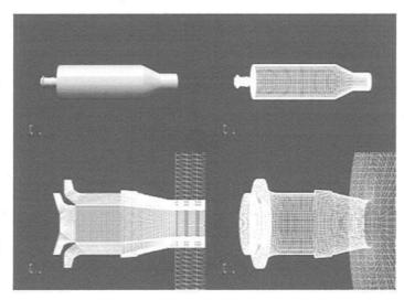
Figure 2: Mesh generated for the case (up) and inlet detail (down) for mesh.
