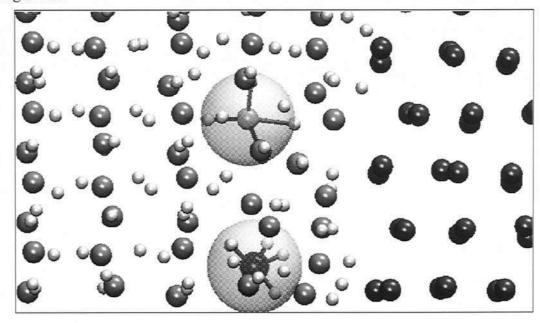
Figure 2: Snapshot of the  $MgH_2$ -Mg interface with Fe in POS2 at T=500 K. H atoms are in white, Mg atoms are in light ( $MgH_2$  side) and dark (Mg side) grey and Fe atom is in black. Large transparent circles are used to indicate the first H-shell of an Mg atom (up circle) and of the Fe atom (bottom circle). These circles enlighten the different first-shell coordination of the two atoms.
