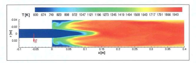
Figure 5: Average temperature field obtained with the POLIMI chemical mechanism.
