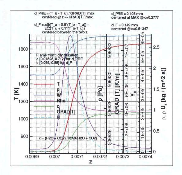
Figure 4: One-dimensional flame predicted by the POLIMI mechanism.
