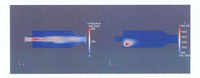
Figure 4: Results of simulation: cold flow (left) and reactive flow (right).
