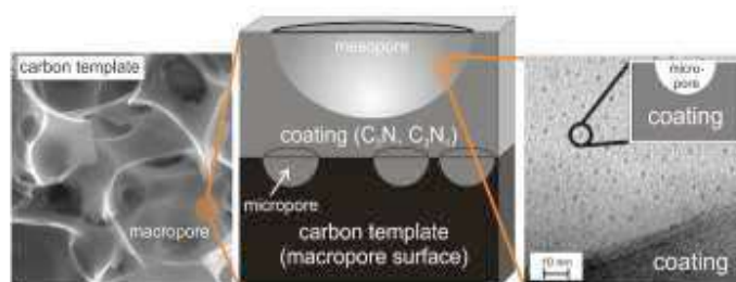
Fig. 1: Electron micrographs of the carbon template, the micropores and the coating of N-doped graphene
