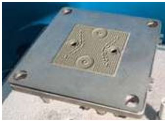
Fig. 2. Left: Interconnect (for 52x52mm cells) with square design with NiO paste painted on it. Right: Interconnect for rectangle shapes cells (76x60 mm).
