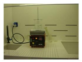
Fig. 4 - Heated etch bath (NaOH)
