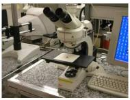
Fig. 5 - System for tracks count
