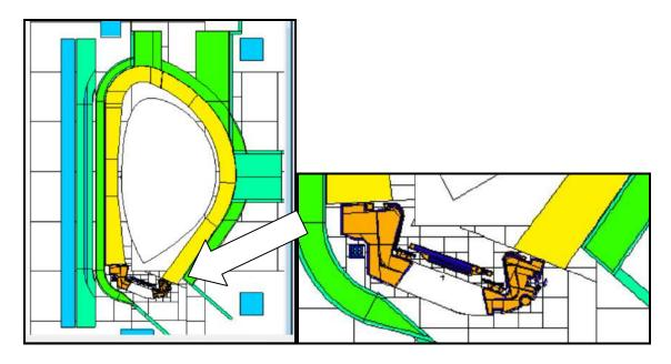
Fig.1: MCNP model of DEMO 2017 with integrated heterogeneous divertor model based on 2019 design
