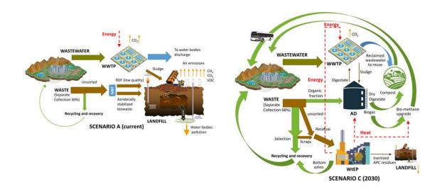
**Figure 1**. Scenario A- Current and Scenario C- Future (the Waste-Wastewater-Energy Nexus through Industrial Symbiosis). Scenario B is similar to Scenario A except for the percentage of separate collection which is 68% instead of 30% and for the MBT which is not present in scenario B. (Modified from Mancini et al., 2022 [12])
