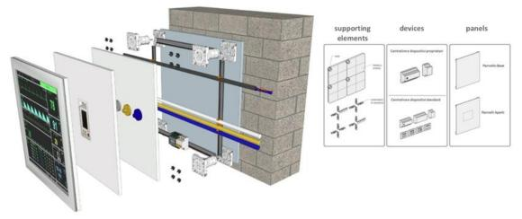
Figure 2. Stratigraphy and technological levels (Support, Plants, Panel)
