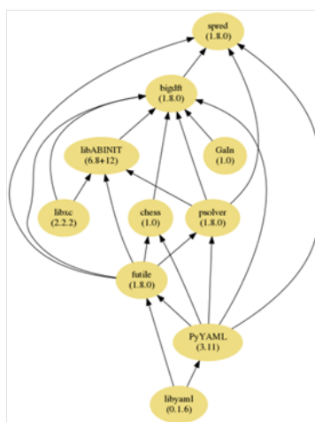
Figure 3: Scheme of the BigDFT modularity. Modularity of the numerical codes improves the sharing of codes, their management, their maintainability and their optimization for HPC platforms.
