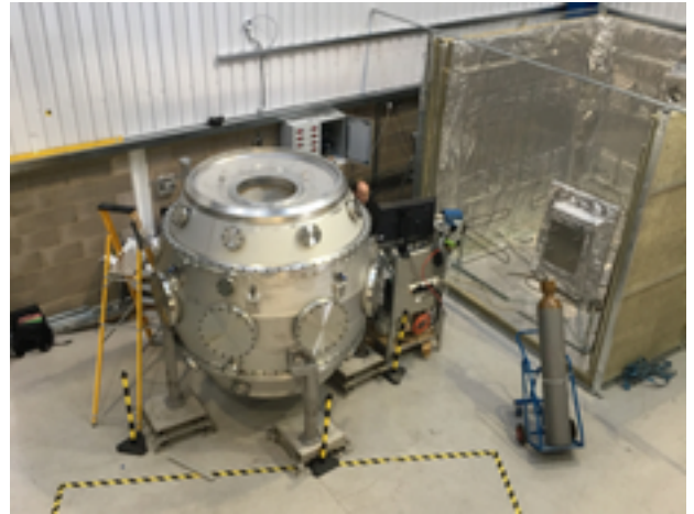
Fig. 2. Photos of the centre post of the device (left) and the entire ST40 inner vacuum chamber (right) ready to be baked in the baking stove
