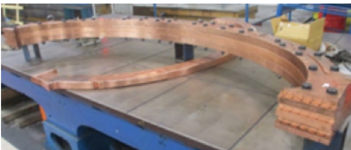
Fig. 3. Photos of a copper TF return limb (top) and of the entire centre post with its 24 TF wedges (bottom).
