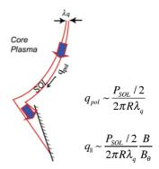
Figure 4. How to cope with large values of the power flux on the divertor: geometry helps, but by itself is not sufficient to handle a heat flux probably higher than that on the sun surface.
