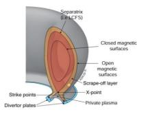
Figure 2: Plasma edge: geometry of the Scrape-Off Layer (SOL) and of the divertor plates.
