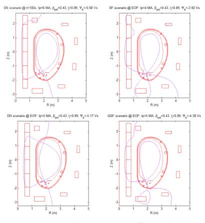
Figure 5: Conventional and alternatives magnetic configurations that can be realized by the DTT poloidal field system.
