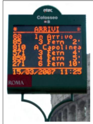
Figure 3.7: Predicted bus arrival times at electronic bus stop
