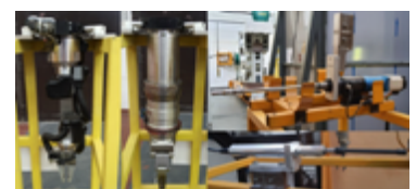
DRP hall – end effectors and bolting tools
