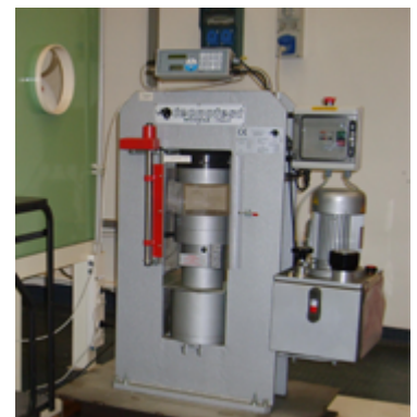
Apparatus to test the specimens compressive strength
