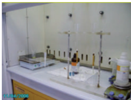
RP Saluggia – Radiochemical treatment of bioassay samples for Plutonium radioisotopes determination and electrodeposition apparatus
