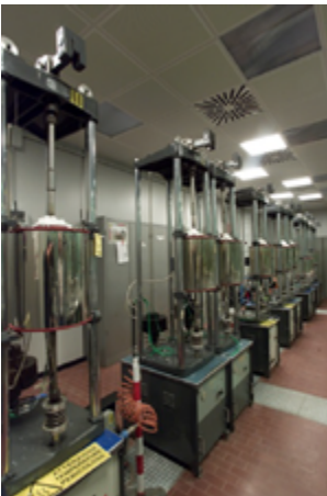
CREEP laboratory overview, tensile and bending
