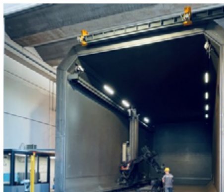
Vacuum chamber (left) of the EBW machine and soldering robot (right)
