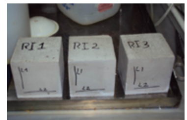
Concrete specimens for qualification tests
