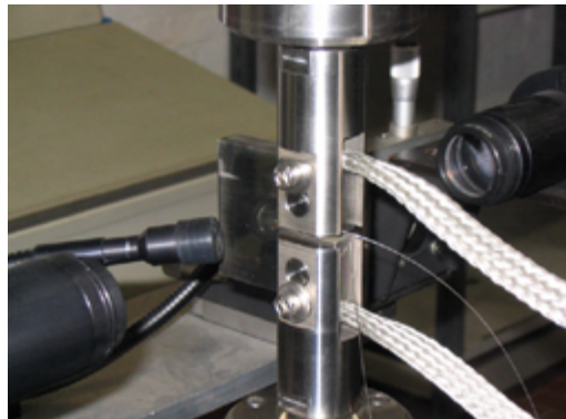
High temperature fracture toughness test and Fatigue crack growth test
