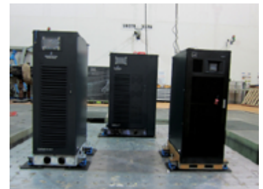
Dynamic/functional tests on UPS systems
