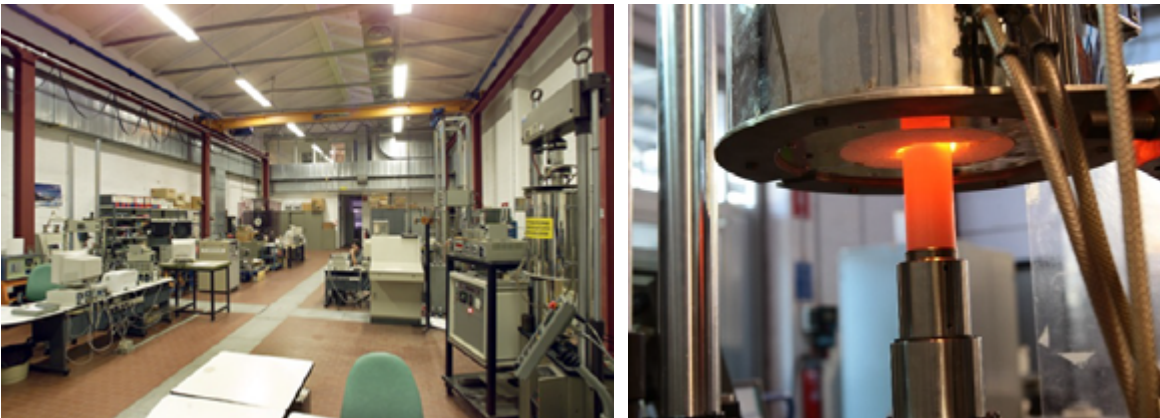
Overview MTS laboratory and MTS 50 kN machine with oven detail
