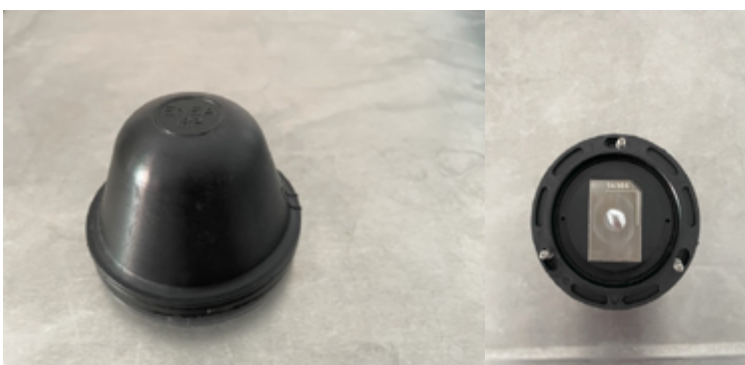
Alpha track radon passive sampling deviceV
