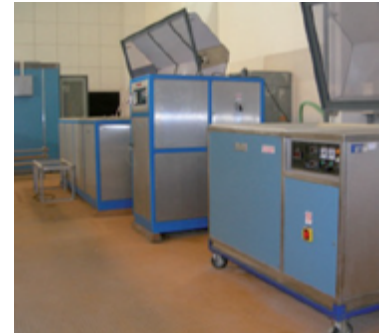
Climatic chambers and salt spray chambers for environmental qualification of nuclear components and systems
