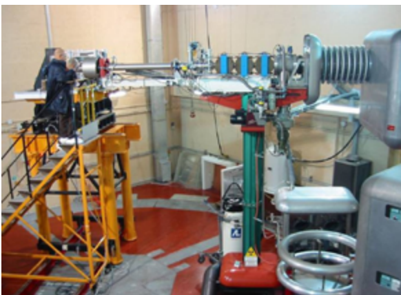
RadHard testing of FBG sensors at the Frascati Neutron Generator plant (ENEA – Frascati Research Centre)
