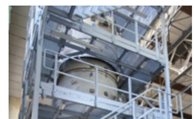
Helical coil steam generator mock-ups for heat transfer and FIV tests (NuScale Power SMR)
