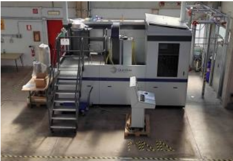
Hot isostatic press and Mo furnace detail
