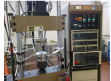
MTS universal testing machine 100 kN size
