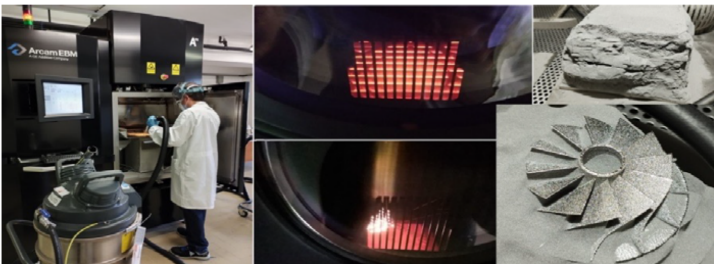
3D printing by EBM process with representative pictures of the extracting phase by sandblasting process of the components; (DX) Mock up (1:4 Scale) of the 3D printed Ti6Al4V handling hinge for Demo Divertor process
