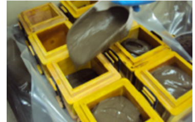
Preparation of cement mixture and packing of specimens
