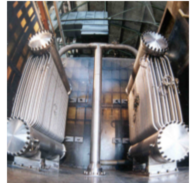
Thermo-mechanical tests on decay heat removal systems of LWR reactors (GE SBWR reactor, PCC: 10 MW, 175 m 3 )
