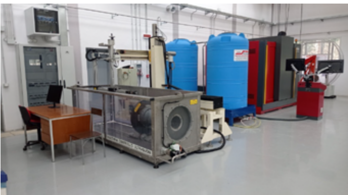
Technological Hall in the foreground ultrasonic tank for aerospace components
