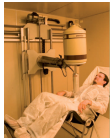
Whole Body Counter – In vivo measurements for internal radioactive contamination
