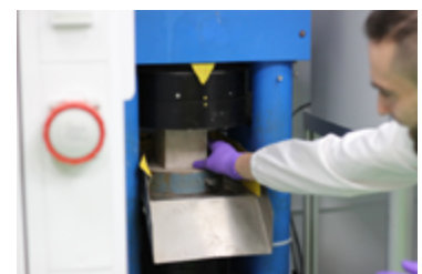
Compressive strenght test
