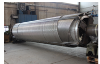
Dry-out tests on a rod cluster of a BWR reactor (10 MW; 70 bar)
