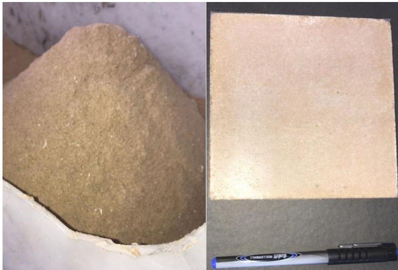
Figure 1a. MDF and Chipboard Powder; Figure 1b. Pre-Prototype Panel
