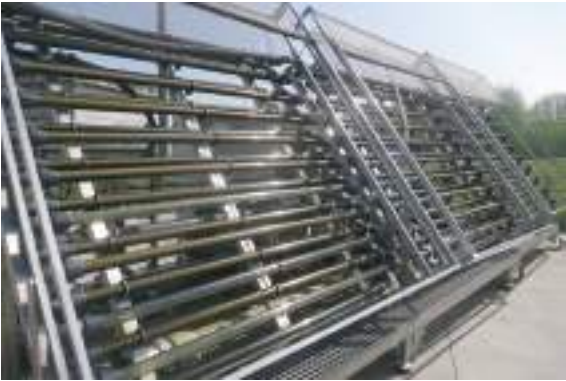
Fig. 4. SOFCOM process: photobioreactor arrays.
