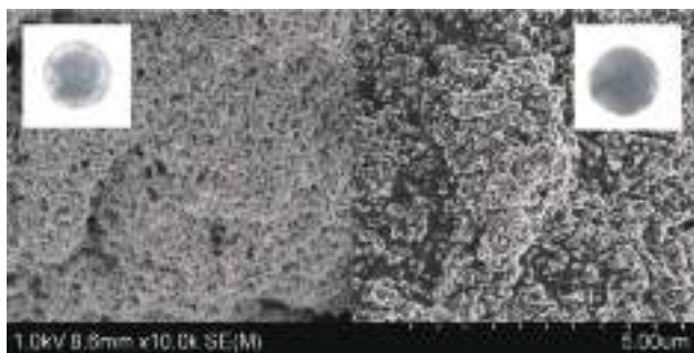
Fig. 2 – SEM image of newly prepared electrodes, 70% \text{H}_2\text{O} (left) and 40% \text{H}_2\text{O} (right). Insets: Macroscopic photo of the electrodes (11 mm diameter).
