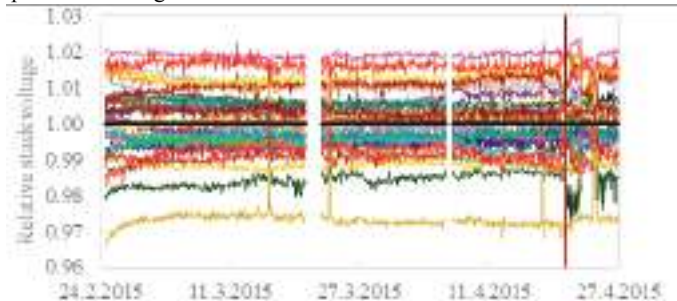
Fig. 1. Stack voltages relative to the average voltage (black line) during the test period. Different colors represent different stacks.
