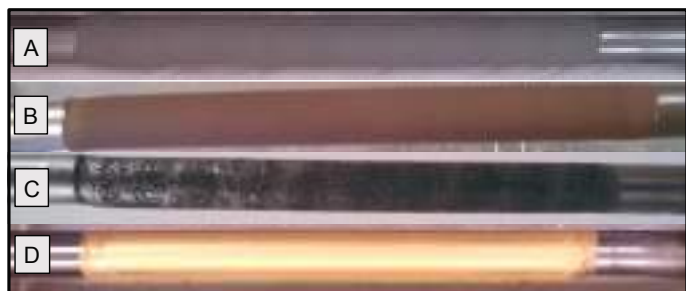
Fig. 1. Fabrication Steps: [A] Initial support [B] Oxidation at 500°C [C] Grading [D] Final Pd-Au metallic layer
