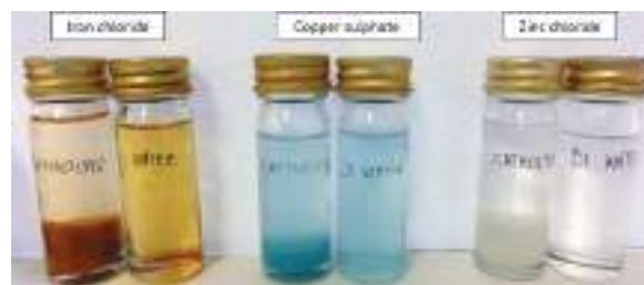
Fig. 3 Precipitation of heavy metals from the exposure of samples to MFC-generated catholyte
