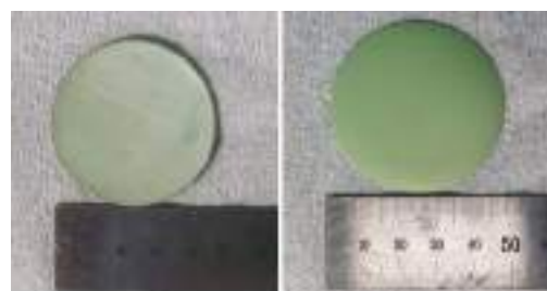
Fig. 3. Large-area anode-supported electrolyte with a diameter of 50 mm fabricated by co-tape casting process.
