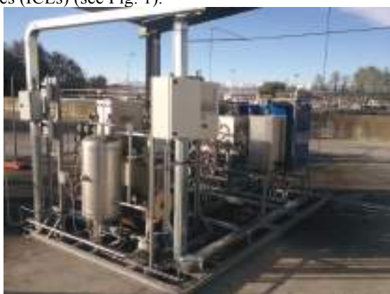
Fig. 1. The SOFCOM plant in the SMAT WWTP of Torino, IT (the fuel cell section of the plant is shown with BoP, gas clean-up unit, reformer, oxycombustor and anode exhaust condenser).
