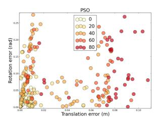
Fig. 8. Recognition error caused by occlusion: legend information indicate occlusion percentage
