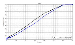
Fig. 10. Ring probability distribution with one static target. Plot of success rates vs. detection ranges. On the right the same plot but with a logarithmic scale (LF, black continuous, RW, blue dotted).
