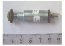
Fig. 1 Miniature in-tube robot.
