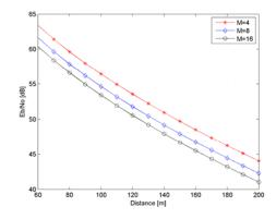
Fig. 3. Eb/No versus distance for different M-FSK modulation formats.
