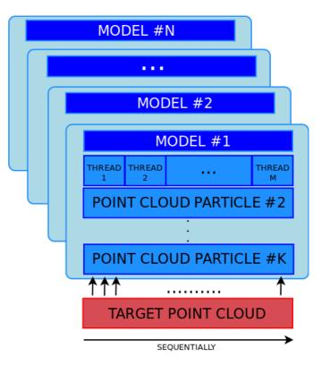
Fig. 5. Parallelization of fitness function computation on CUDA architecture: while the points of the target are confronted serially, the point clouds of i-th model are subdivided on more than one thread.
