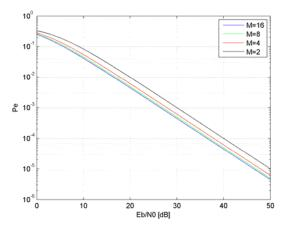
Fig. 2. Bit error probablility versus  $E_{\text{b}}/N_0$  in RFC channel for M-FSK modulation.
