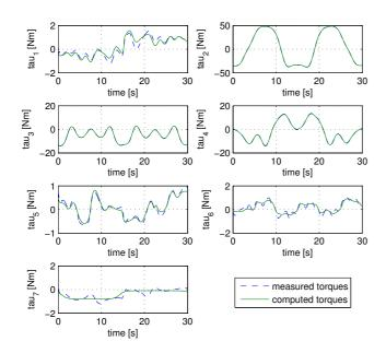
Fig. 1. Comparison between the measured joint torques  $\tau_J$ , as retrieved from the KUKA LWR robot, and the joint torques  $\hat{\tau}_J$  computed from (1) (in the absence of external torques,  $\tau_{ext} = 0$ ) when using the identified dynamic coefficients, including friction. The robot is performing a generic motion not used during the identification (validation phase).
