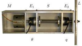
Figure 3. The SEA prototype used as testbed. The motor M is connected to the torsional spring S and the angular quantities  $\theta_m$  and  $\theta_e$  are measured by encoders  $E_1$  and  $E_2$  respectively.
