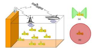
Fig. 1. Swarm system model with optical (a case) and acoustic (b case) communications.
