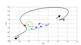
Fig. 9. From the blue square the target (the red point) follows the curve, while the search starts from a random point, in this case close to the Origin. The green dotted circle represents the detection sensor range. The arrows indicate the motion direction of the single target.
