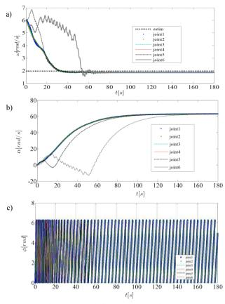
Fig. 8 – Adaptive CPGs oscillators parameters dynamics: a) frequency; b) amplitude; c) phases
