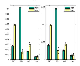
Figure 5. RMS and maximum torque tracking error for passive PID, passive PD (tuned for the low impedance), AB and AD controllers in high (green) and low (yellow) impedance conditions. Three- $\sigma$  confidence intervals are shown.
