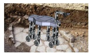
Fig. 1 A 3D simulation of hexapod robots in survey activity
