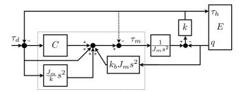
Figure 2. SEA force control schema relative to equation (10) with  $k_b < 1$  to prevent feedback inversion. The dotted arrow represents motor backdrivability.
