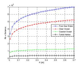
Fig. 6. Bit Rate distance product in function of transmitter power different types of water.
