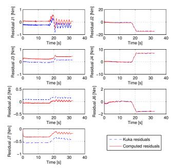
Fig. 2. Comparison between the KUKA FRI output  $\hat{r}_{num}$  and the residual  $\hat{r}$  computed from (2) with the identified dynamic model coefficients. The robot performs first a rest-to-rest motion without payload for about 18 s (residuals should remain at zero). Then, a suspended payload is hung at the end effector, which is detected as an external torque  $\tau_{ext}$  (oscillations are due to the slight swinging of the payload).
