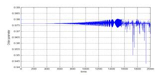
Fig.15. The order parameter  $\Phi(t)$  time series oscillates around 0.96. The small *k* produces the loss of synchronization visible after t=1600 time units.
