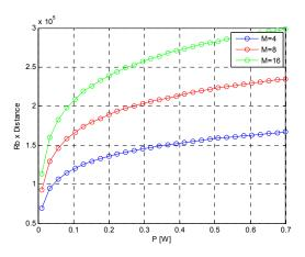
Fig. 4. Bit Rate distance product in function of transmitter power for different M-FSK modulation formats.
