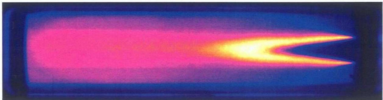
*Figure 3: Averaged OH field obtained by using 400 OH-PLIF samples.*
