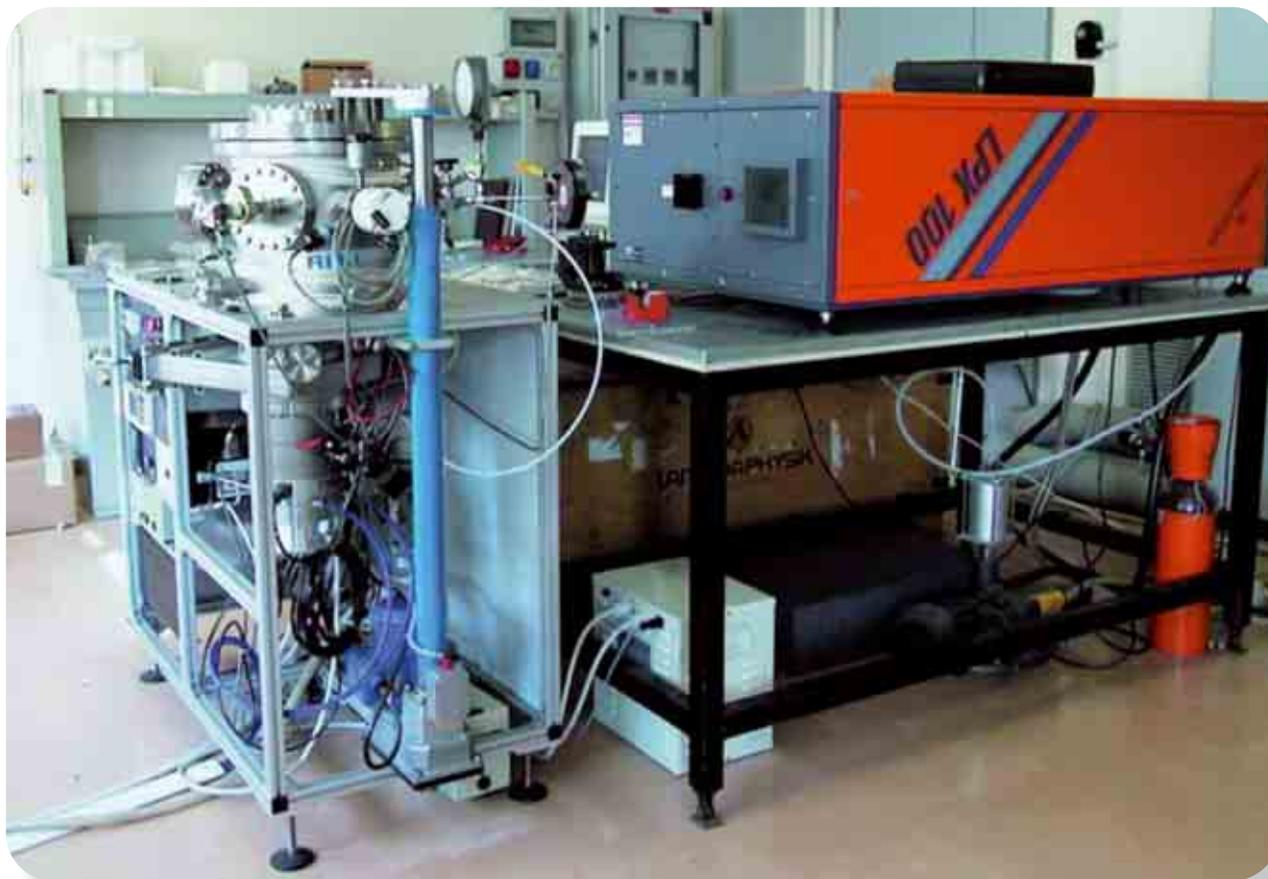
Impianto per Pulsed Laser Ablation con laser a 100 Hz/150 mJ.
