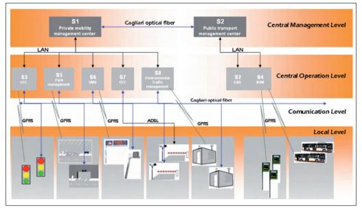
Figure 3.39: Telematics platform architecture
