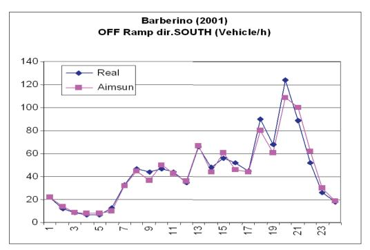
Figure 4.17: Comparison between simulated and observed traffic flows at the Barberino off
