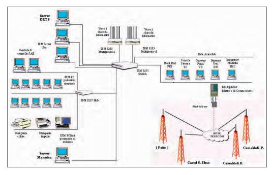
Figure 3.24: Overall architecture of the AVM system operated by ANM in Naples
