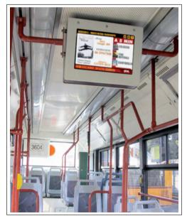
Figure 3.10: MOBY service LCD screens providing real-time travel information to passengers
