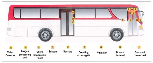
Figure 3.53: Architecture of on-board devices
