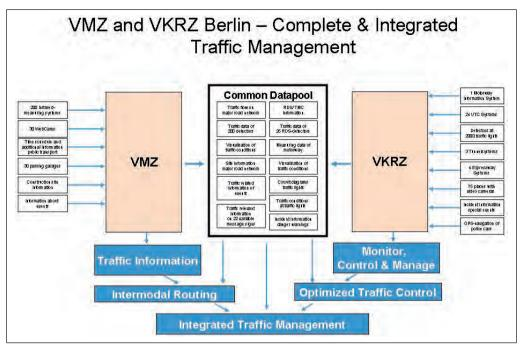
Figure 3.22: Interfaces and interaction between VMZ and VKRZ
