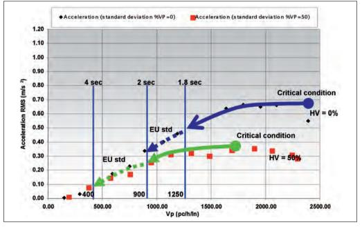
Figure 4.29: Safety thresholds for traffic flows inside tunnels
