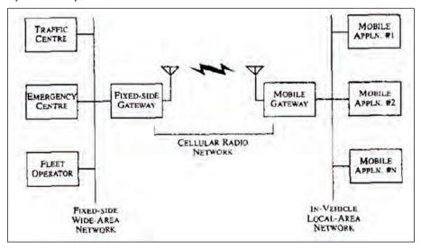
Figure 5.3 The SOCRATES reference architecture (Source: Zijderhand and Biesterbos, 1994)
