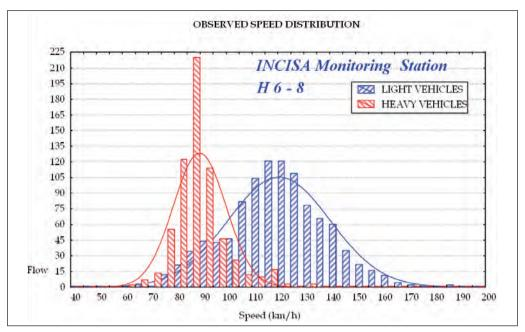
Figure 4.16: Observed actual speeds in two non-peak hours at the traffic monitoring station of Incisa.
