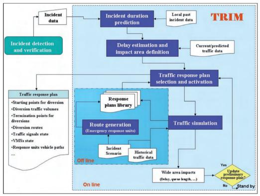
Figure 5.13: Flowchart of TRIM basic functions
