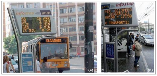
Figure 3.25: On-street public transport user information: Infostop panels in Naples showing (a) estimated bus arrival times and (b) service disruption information
