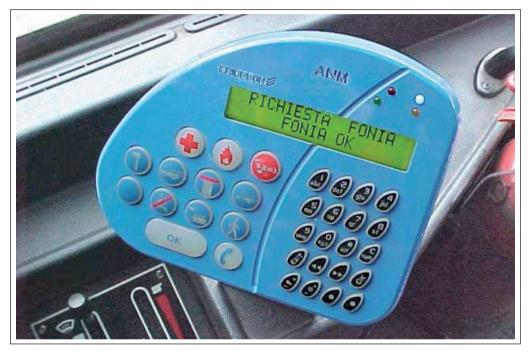
Figure 3.29: On-board driver terminal in ANM AVM system
