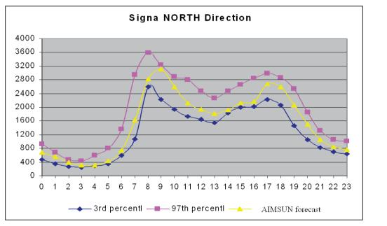
Figure 4.18: Observed hourly traffic flows in North direction at the Signa detector vs. simulated by AIMSUN 197
