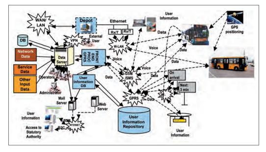
Figure 7.1: Architecture of an AVM system based on GPRS long-range communication system
