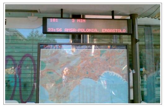
Figure 3.26: On-street public transport user information: electronic information displays at bus stop shelters in Naples
