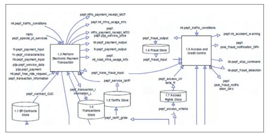
Figure 2.1: Example of Data Flow Diagram: part of FRAME Functional Area "Provide Electronic Payment Facilities" (source: KAREN / e-FRAME project, <u>http://www.frame-online.net</u>)
