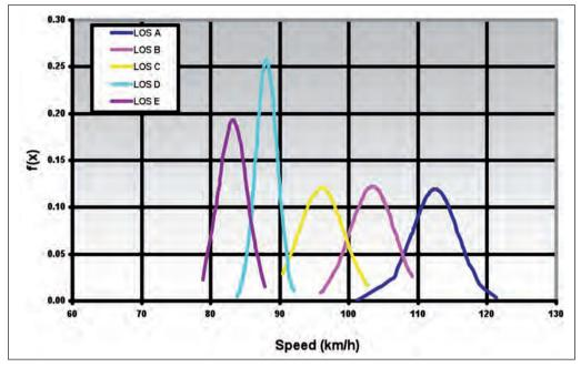
Figure 4.26: Speed distribution (%HV=0)
