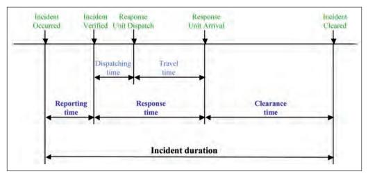
Figure 5.5: Components of incident duration
