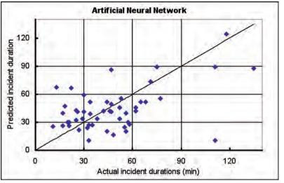
Figure 5.9: Neural Network prediction results versus duration test data
