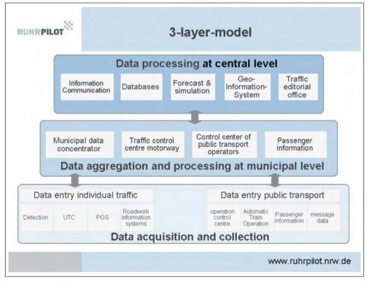
Figure 4.8: Ruhrpilot's multi-layer system architecture
