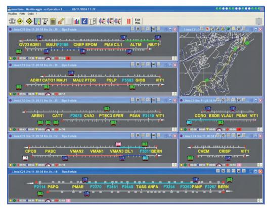
112 Figure 3.27: Display of lines data and service regulation in the AVM Control Centre
