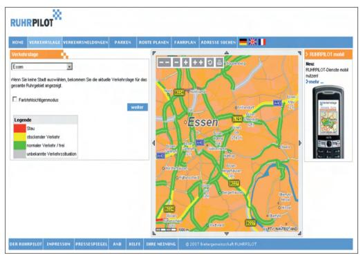
Figure 4.6: Traffic conditions and routing information available from the web-site "www.ruhrpilot.de"
