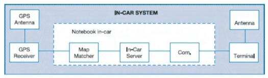
Figure 5.2: Block scheme of single car equipment in C2CC
