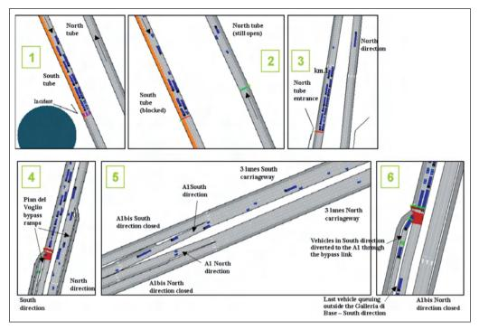
Figure 4.21: Modelling of some of the main incident management phases
