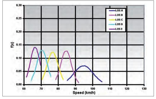
Figure 4.27: Speed distribution (%HV=50)
