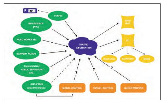
Figure 3.2: Relationship between the different ITS systems and information available on the Trafikinfo webpage. The integrated system is the Strategic Traffic Management System of Aalborg
