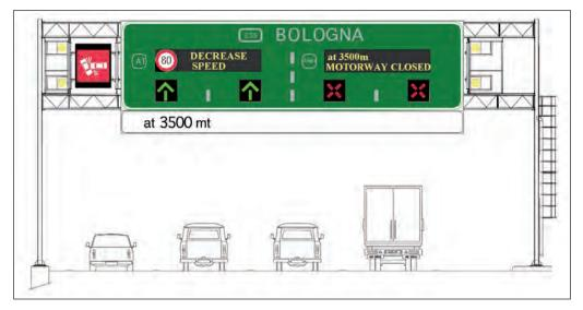
Figure 4.19: Hypothesis of special VMSs with lane access control before the beginning of the A1bis
