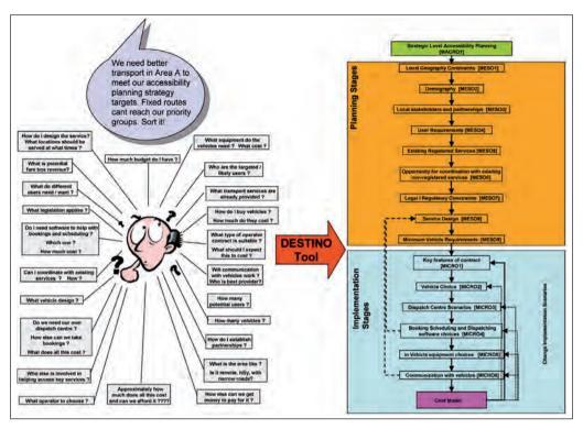
Figure 6.1: The DESTINO Tool Design Framework
