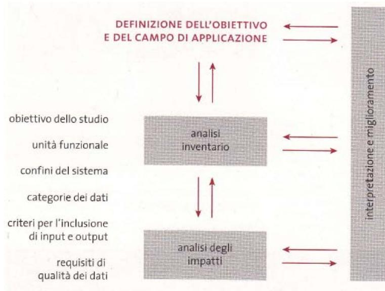
Figura 2: Schema operativo Fase 1 LCA "Goal and Scope Definition"
