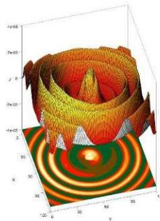
**Numerical results for the electromagnetic field emitted by the Jay-Beam 7276 antenna**
