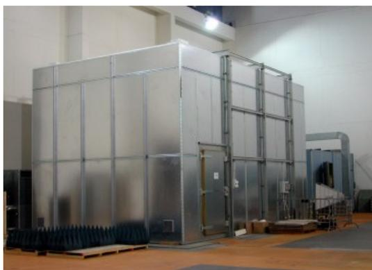
The **VECUVIA** semi-anechoic chamber is the main test facility of the ENEA Laboratory of Electromagnetic Fields performing **electromagnetic compatibility** tests and measurements at a 3 m distance from antennas. Its external dimensions are  $(9.00 \times 6.00 \times 5.60) \text{ m}^3$ .
