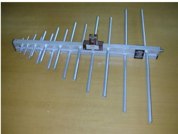
**Log-Periodic Dipole Array Antenna (LPDA)**
