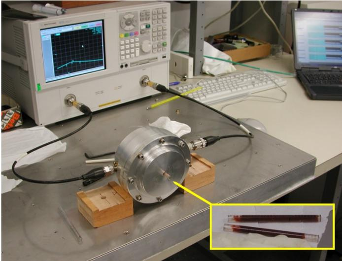
As an example, the side picture shows the experimental setup to measure the **electric permittivity  $\epsilon$**  of steer liver (in quartz tubes) by using a cylindrical resonant cavity.
