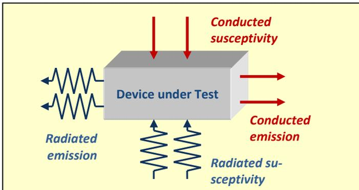
On demand by external customers, both public and private, the Laboratory of Electromagnetic Fields performs electromagnetic compatibility tests on electric and electronic devices and systems.
