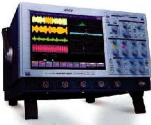
Moreover, the laboratory is equipped with a **LeCroy WaveMaster 8500 digital oscilloscope**, which is able to sample signals at a maximum speed of 20 GS/s up to 5 GHz. This instrument is used to characterize waveforms and pulses with high frequency content.
