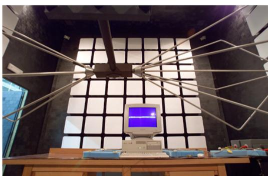
Rotating the device under test and modifying, at the same, time the elevation and polarization of the antenna mounted on the mast made it possible to identify the maximum emission configurations as required by some important electromagnetic compatibility standards (**EN 55022**, **EN 55011**).
