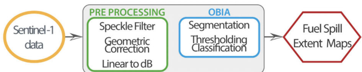
Figure 3. Flowchart showing the methodology of the fuel spill extent delineation by means of the Sentinel-1 images
