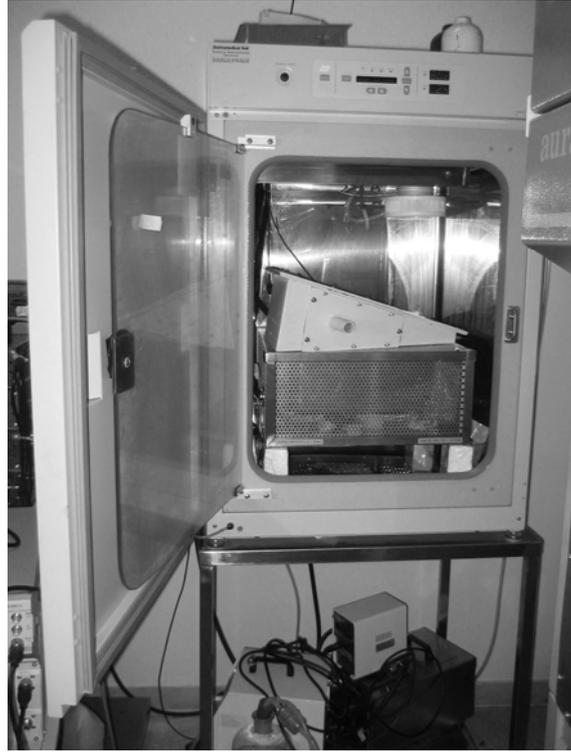
Figure 1 - GTEM cell prototype in the incubator
