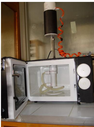
**Figure 3 - Reactor featuring simultaneous US/MW irradiation (fused-quartz horn)**
