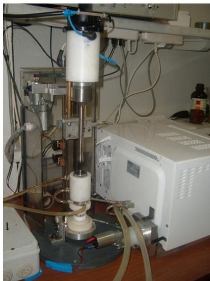
Figure 1 - Flow US/MW reactor (first prototype for sequential irradiation)
