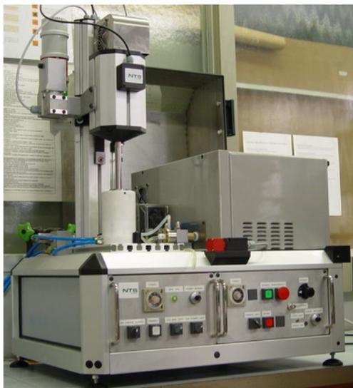
**Figure 2 - Professional Flow US/MW reactor**
