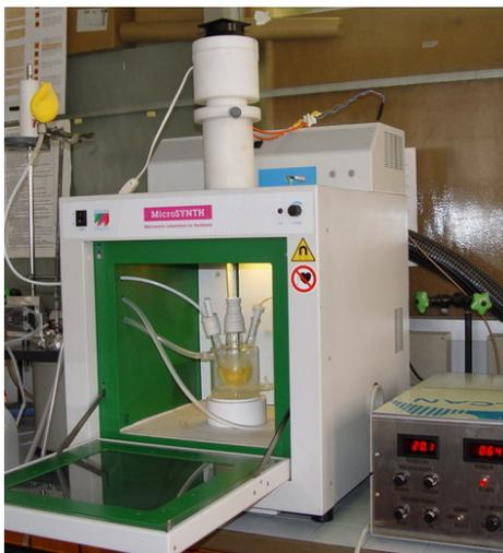
**Figure 4 - Combined US/MW (pyrex horn) with cooled reaction vessel**
