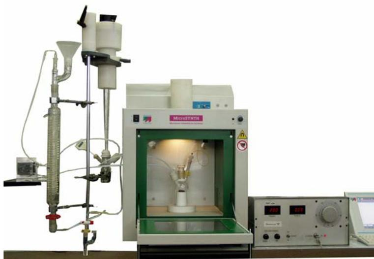
**Figure 6 - Double set up US/MW reactor: 1) Sequential Flow System or 2) Simultaneous US/MW irradiation**
