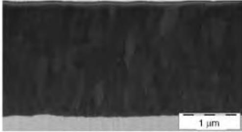
TEM lamella obtained by FIB milling and thinning. In-situ SEM-FEG observation (SE, 5 KV), 12000x
