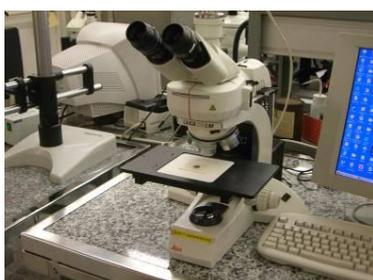
Fig. 5 - System for tracks count
