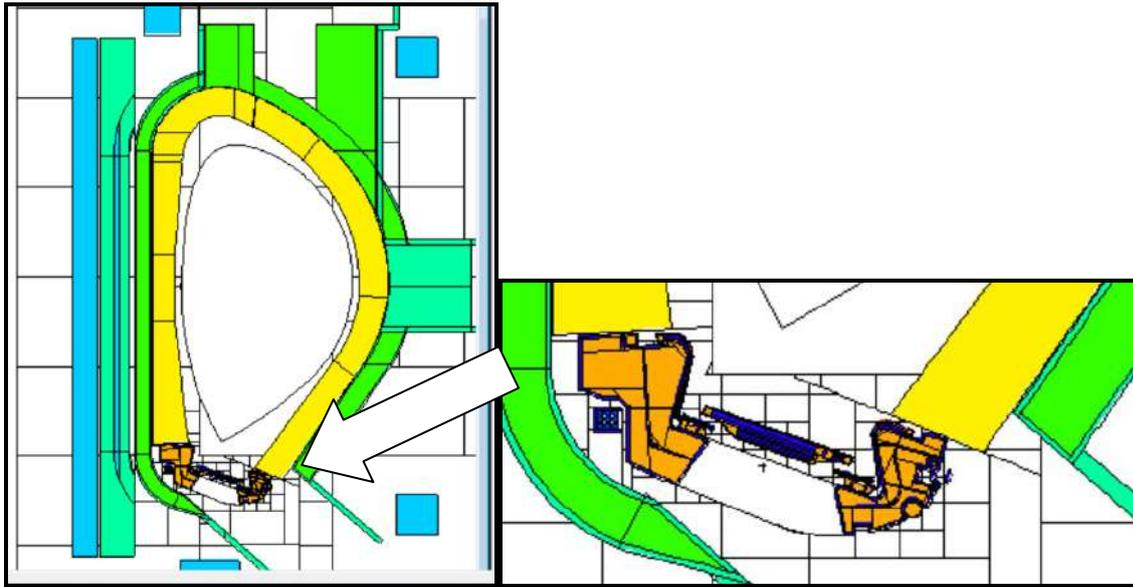
**Fig.1:** MCNP model of DEMO 2017 with integrated heterogeneous divertor model based on 2019 design
