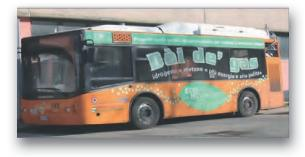
Within the framework of the **LIFE+MHYBUS** European Project managed by the Emilia Romagna Region for reducing consumption and emissions of local public transport, ENEA has been involved in research and experimentation on -methane-hydrogen mixtures, an internal combustion technology that has proved to be very promising.
