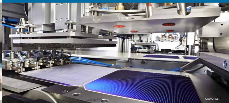
industrial HJ technology with the objectives of more than 23% mean efficiency for cell and more than 400Wp power for module.
