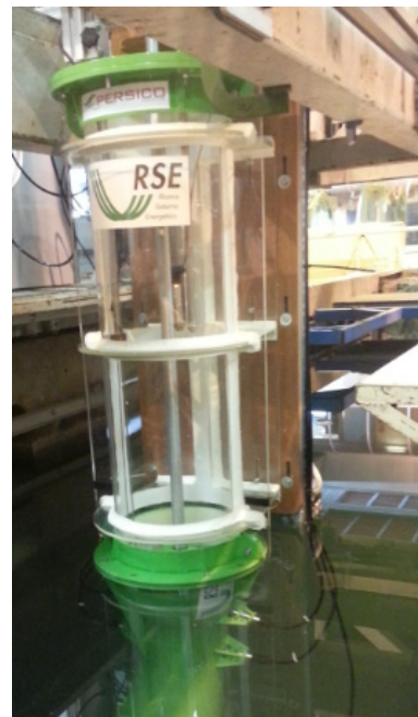
Figure 7 - The WAVESAX 1:5 scale prototype
