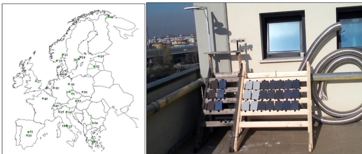
Figure 8.1 – Map of test sites of the monitoring programme of ICP Materials (left) and test site in Venice with material samples on the rack (right).
