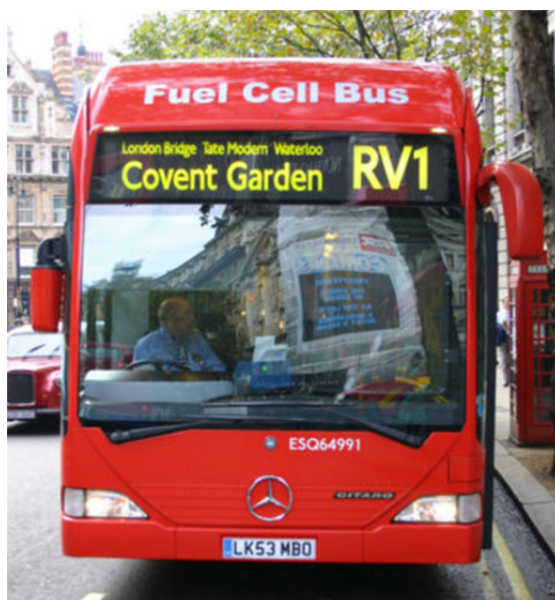
FIGURE 19 London bus on the RV1 line, powered by Ballard FC Velocity-HD6 PEMFC modules delivering 150 kW 6
