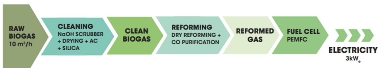
FIGURE 30 Flowchart of the PEMFC integrated pilot system in Murcia
