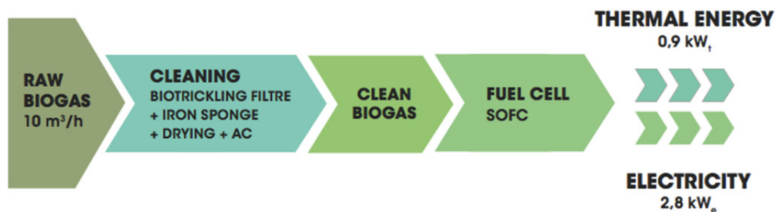
FIGURE 29 Flowchart of the SOFC integrated pilot system in Mataró
