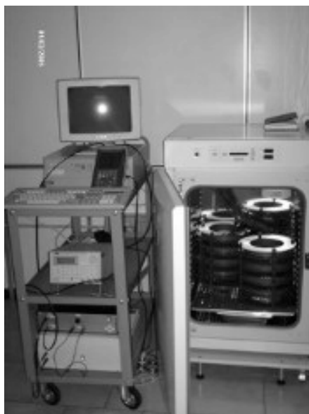
Fig.3. ELF exposure system designed and realized in cooperation with the Department of Physics, University of Bologna. It allows double blind exposures of biological samples. Helmholtz coils are hosted inside a cell culture incubator
