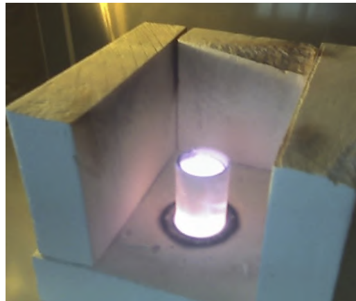
Fig 6 Specimen melting in crucible in MW oven
