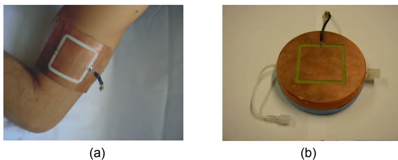
Fig. 9. Flexible applicator (a) and applicator with bolus (b) for physiotherapeutic MW hyperthermia
