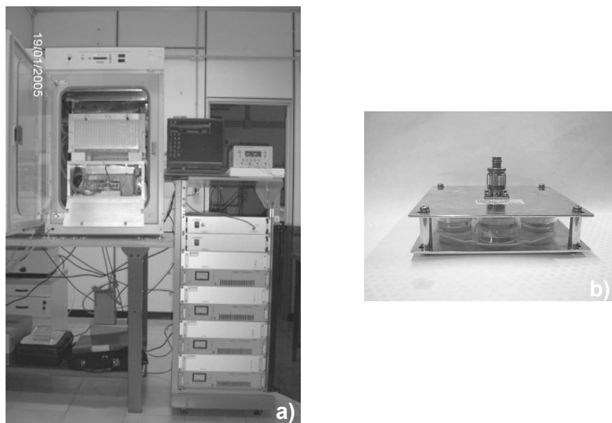
Fig. 2. (a) Exposure system for cell cultures operating in the frequency range of 895-905 MHz. It employs four WPCs as exposure chambers and has been designed and realized in cooperation with the Section of Toxicology and Biomedical Sciences of ENEA-Casaccia (Rome) in the framework of a project funded by Cellular Telecommunication and Internet Association (CTIA), with the scientific supervision of the US Food and Drug Administration; (b) WPC hosting four biological samples
