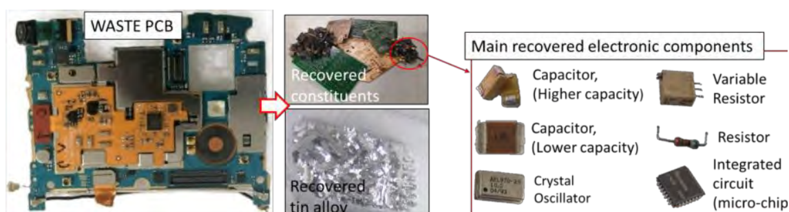
Figure 1. Example of waste PCB and recovered constituents: electric and electronic components, tin alloy and copper layer and fiberglass ply.
