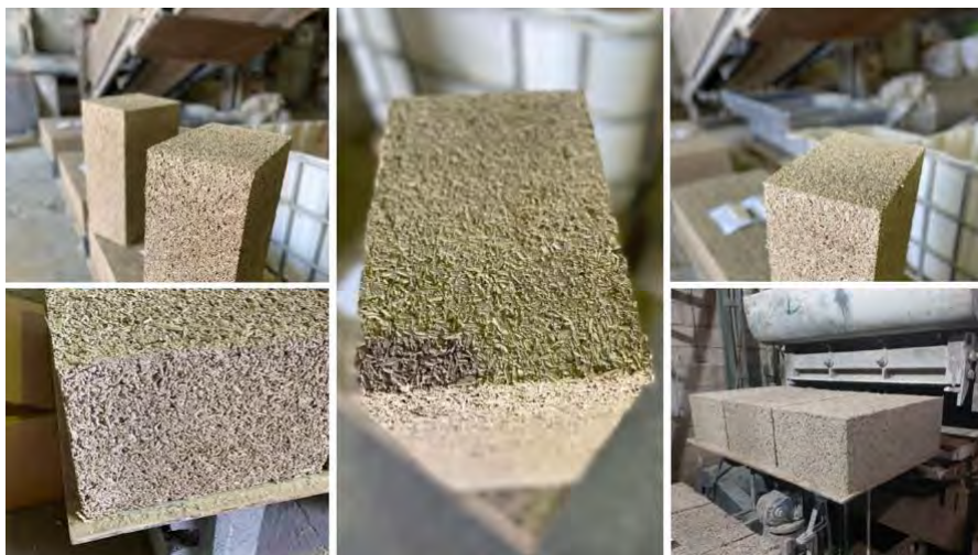
Figure 1. Bio-block prototype produced and test (courtesy of PEDONE Srl).
